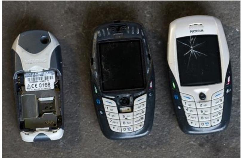
Examples of non-functional mobile phones: missing battery and cover (left), damaged keyboard (mid) and broken screen (right).
