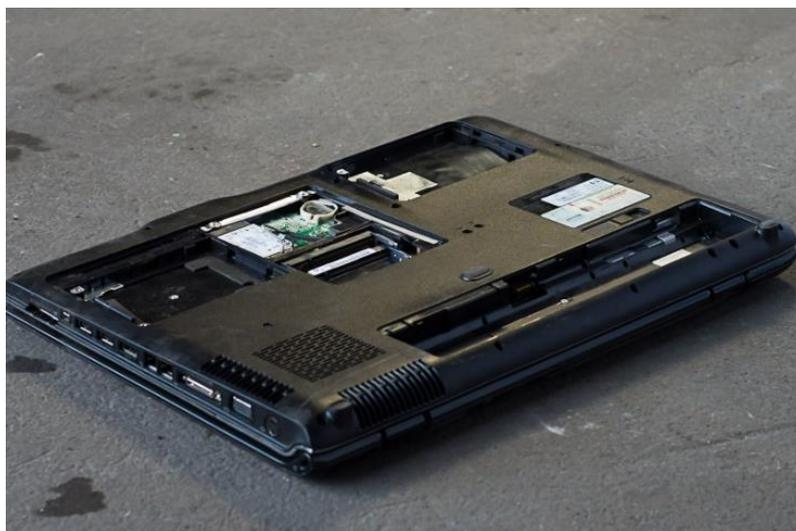
An example of a non-functional laptop computer: battery, hard disk and covers missing.
