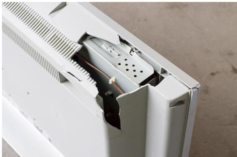
An example of a non-functional flat screen TV: serious damage in cabinet.
