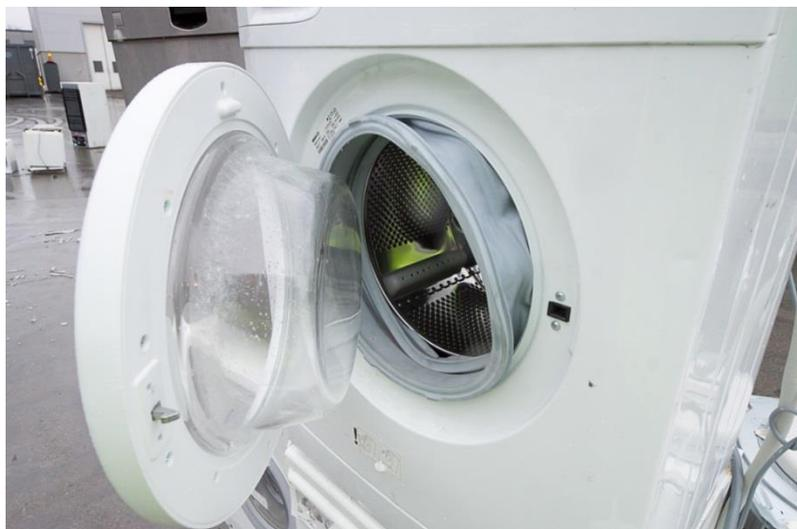
An example of a non-functional washing machine: damaged door seal.
