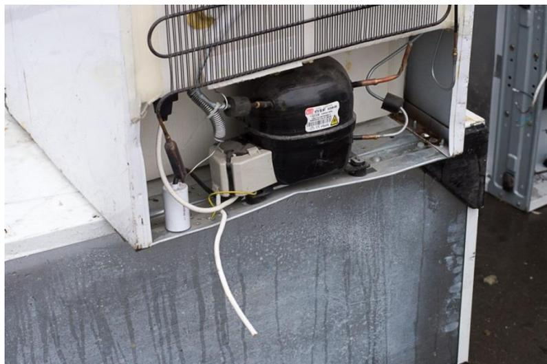
An example of a non- functional refrigerator: power -plug missing.
